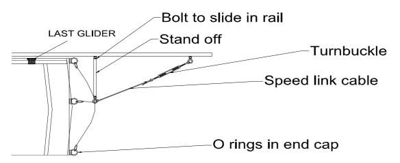
With the Halo suspension system sections can be taken down and washed if necessary without removing the rings. The diffuser has a zipper every 6' to 10' which makes cleaning easy.
