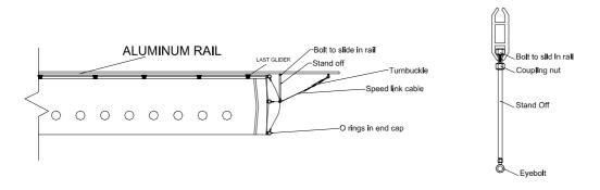
Next slide the nut end of short eyebolt down the rail after the standoff. Then connect the turnbuckle to the eyebolt a speed link cable from the eyebolt of the standoff to the turnbuckle. Make sure the turnbuckle is fully open. Make sure the angle back to the end cap from the eyebolt in the rail is about a 30 degree angle. The eyebolt and the standoff might have to be adjusted to accomplish this. Tighten up the speed link cable.
