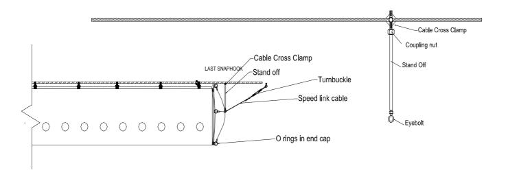
Now you can tighten up the turnbuckle to pull tension on the diffuser. Make sure the worm gear band at the beginning of the diffuser is tight. The option of screws through the band to the sheet metal collar is recommended. Next, turn off the air handler. The diffuser should look about 80% open or more. If not, pull on the end cap to adjust and tighten up the turnbuckle. You might have to adjust the location of the standoff and end cap anchoring system.
