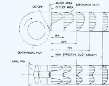
TO CALCULATE 100% EFFECTIVE DUCT LENGTH ASSUME A MINIMUM OF 2-1/2 DUCT DIAMETERS FOR 2000 FPM OR LESS, AND 1 DUCT DIAMETER FOR EACH ADDITIONAL 1000 FPM.
