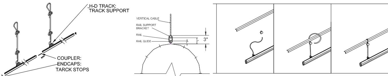
When fabric fittings are incorporated in your installation, align rails with the centerline of the system. All rails must be installed at the same elevation.
