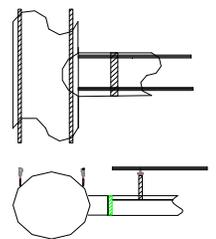
Note: The previous drawings illustrate possible double rail suspension systems. Since every installation is different, support brackets are not supplied. Triple suspension systems used on larger diameters systems
